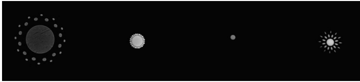
Figure 7: This image shows the circles of confusion for the Imagon with one of its 'sink-strainer' diaphragms in place.
