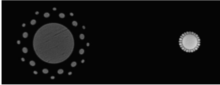
Figure 8: Here's an enlargement of the left two circles of confusion from Figure 7. Note how the two circles of spots surrounding the central opening in the left image have converged to one circle in the right-hand image—clear evidence of spherical aberration. (The striations seen in these images are probably the result of a very slight smeared finger print later discovered on the back surface of the lens.)
