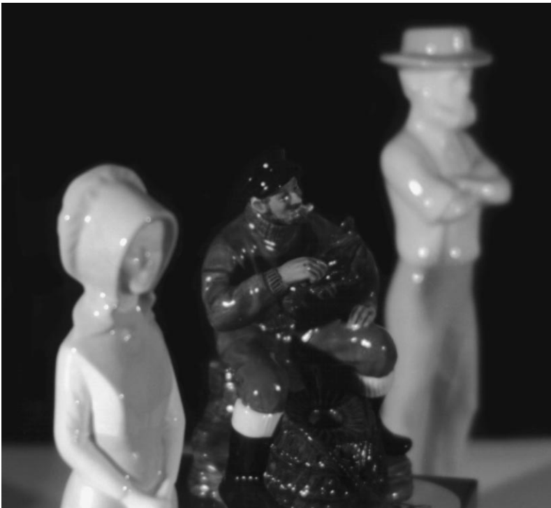
Figure 11: Here's the scene again with the 250 Imagon, using the H=7.7 stop in place. I intended to have to outer rows of sink-strainer holes closed, but there's slight evidence here that one row of holes was open just a tiny bit. Nevertheless, the main effects seen here is the 'bright ring' out-of-focus highlights in the foreground and the 'bright core' highlights in the background.
