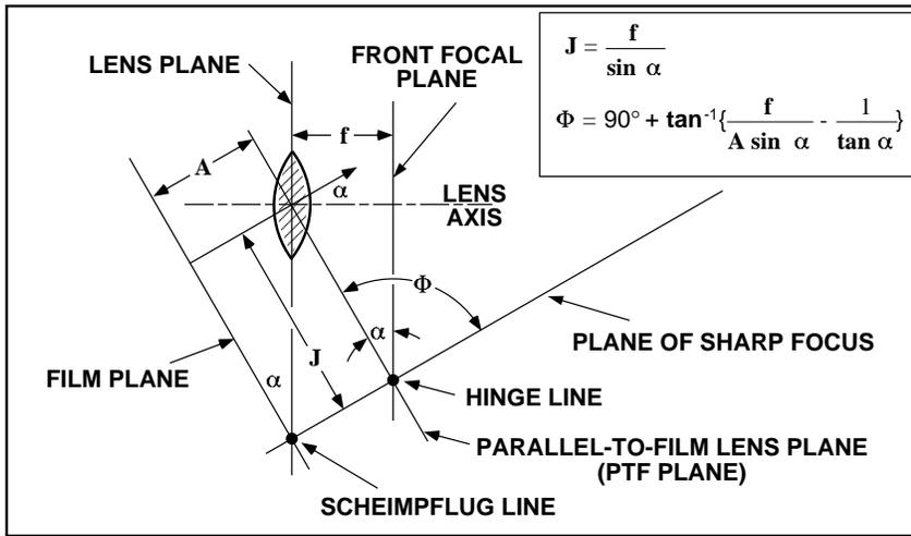
Figure 2: The Scheimpflug rule and the hinge rule combine to provide a complete solution to the view camera optical configuration. The lens-to-hinge line distance,  $J$ , together with the lens focal length,  $f$ , determine the required lens tilt,  $\alpha$ . The lens-to-film distance,  $A$ , and the lens tilt determine the orientation  $F$  of the plane of sharp focus relative to the film plane.
