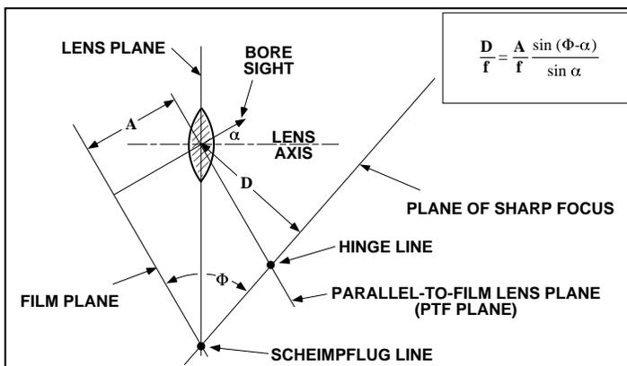
Figure 6: For view cameras, the lens-to-plane of sharp focus distance,  $D$ , is not necessarily measured along the lens axis, as it is for ‘ordinary’ cameras. It is measured in a direction perpendicular to the plane of sharp focus—both for ‘ordinary’ cameras and for view cameras.
