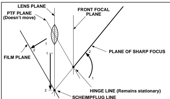
Figure 3: If the film plane is moved closer to the lens, the plane of sharp focus swings away from the lens, rotating on the hinge line. As the film is moved away from the lens, the plane of sharp focus swings up in front of the lens. So long as the angular orientation of the lens plane and the film plane remain unchanged, the hinge line must remain fixed in space.
