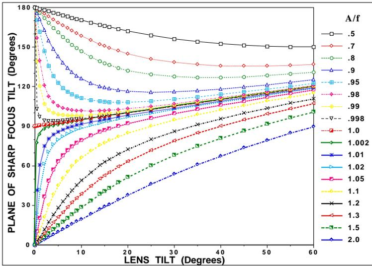
Figure 5: The angle between the plane of sharp focus and the film plane is determined by the lens tilt and the lens-to-film distance. This figure is a graph of plane of sharp focus tilt,  $F$ , as a function of lens tilt,  $a$ , for several different lens-to-film distances. These latter distances are given in focal lengths so that the graph will apply to lenses of all focal lengths.
