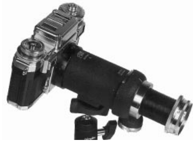
FIGURE 7: With the 2X tube in place, one has the choice of fastening either the "focusing adapter" (lens) or the extension tube to the tripod or copying stand.
