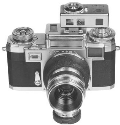
FIGURE 1: Zeiss Contax IIIa fitted with a “Contameter” close-up viewfinder/rangefinder, and the “Contaprox I” 50 mm f/3.5 Tessar macro lens. It’s all set for shooting at a distance of 50 cm.
