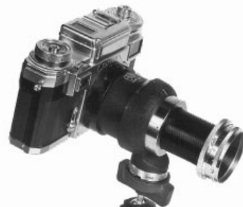
FIGURE 6: Here's the Contax IIIa with Contaprox I and 1X tube: all set for some 1:1 shooting.
