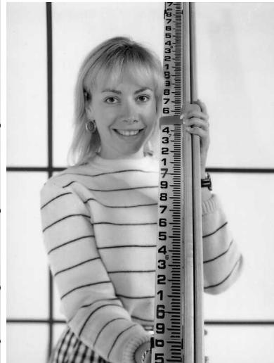
**Example 2:** The survey rod was raised to a higher angular position and the camera back moved away from the lens to focus on the rod in this new position. Again the rod is in focus from end to end. So long as the rod remains hinged at a point 4.2 feet directly below the lens, 7° of lens tilt is the amount required to focus on the rod at any angular position.
